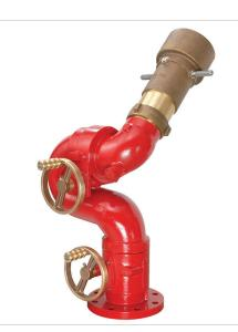
The Angus GMB75 fire monitor is a simple and reliable design with non-reversible worm and wheel gearbox control in both the horizontal and vertical plane. Movement is controlled by dual hand wheels.
